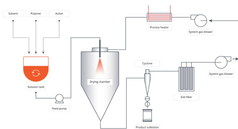
Figure 3: Schematic representation of spray dryer instrumentation configuration.<sup>13</sup>
